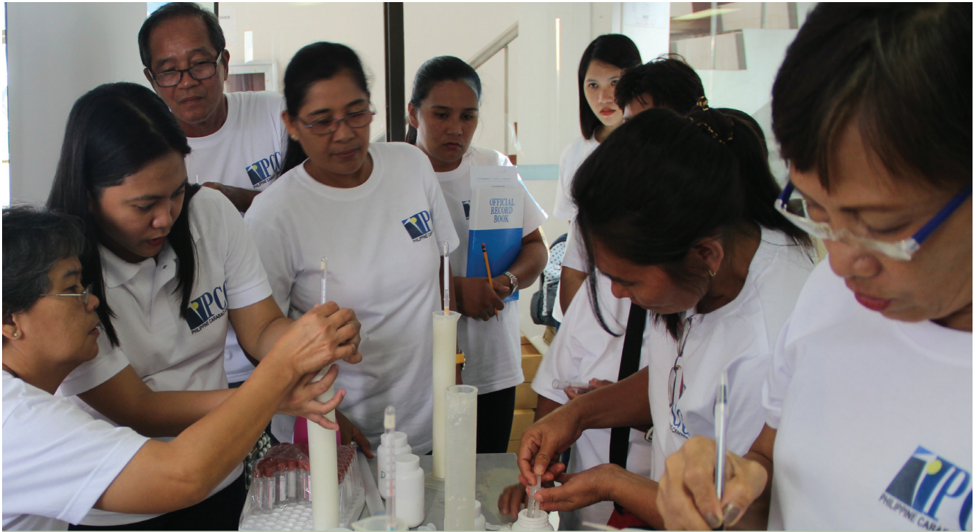
The participants while doing the lactometer test, which is one of the hands-on exercises during the “Refresher Course on Milk Handling and Quality Control.” Lactometer test is performed to find out if the milk is adulterated with water.
