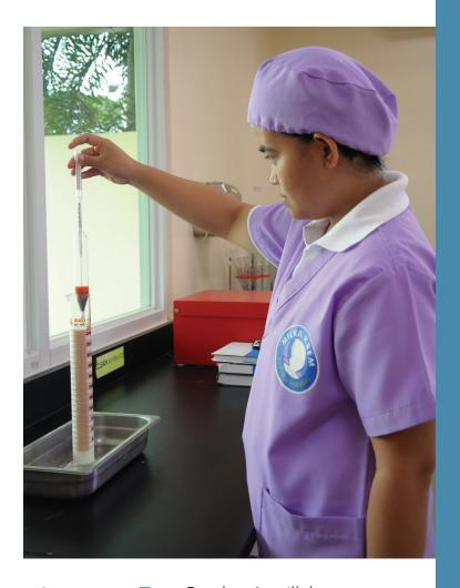
c. Lactometer Test- Carabao's milk has 1.030-1.036 specific gravity. Lactometer test is designed to determine changes in specific gravity, which happen when the milk is adulterated with water or other materials.
